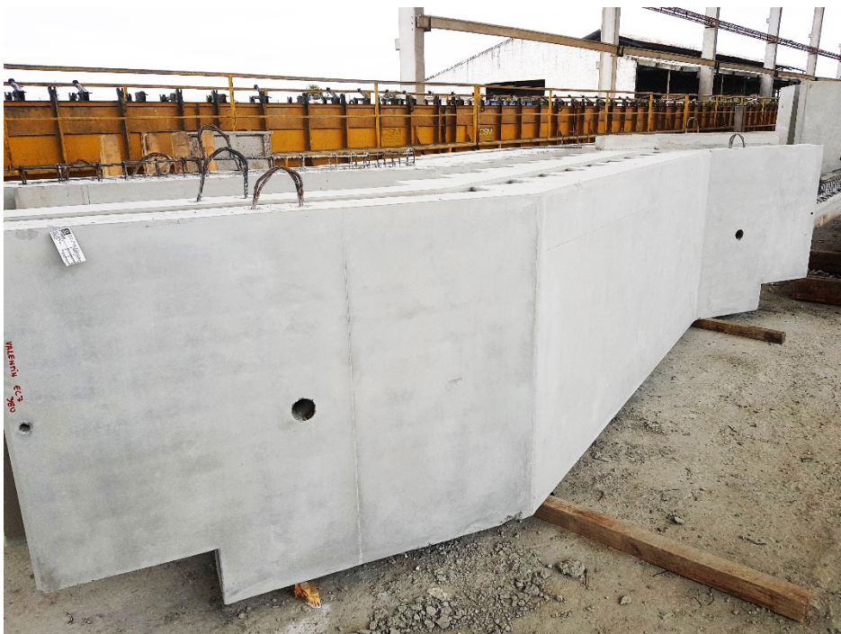
Image 2 The 3-sided fair-faced concrete quality is an important quality feature of precast concrete stairs.
