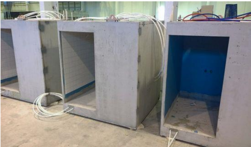
Image 4 All production processes, including sanitary and electrical installations, take place industrially and in a controlled factory environment.
